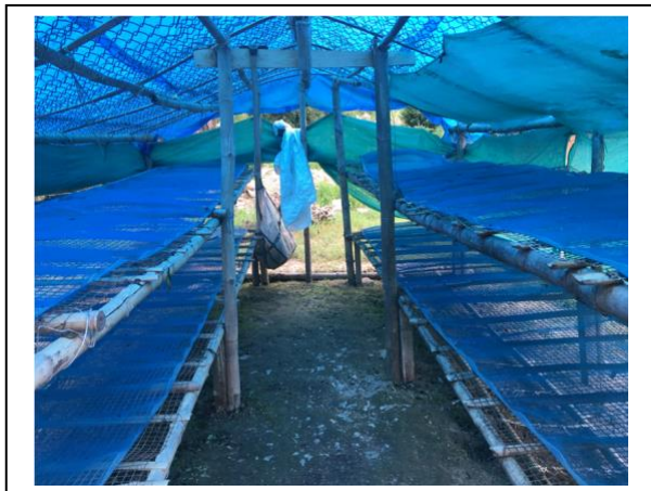
A set-up to dry green tea leaves in a processing unit
